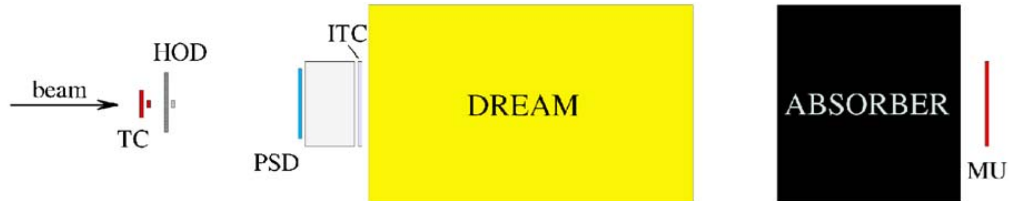
Fig. 4. Schematic view of the experimental setup in the beam line in which the DREAM detector was tested.
