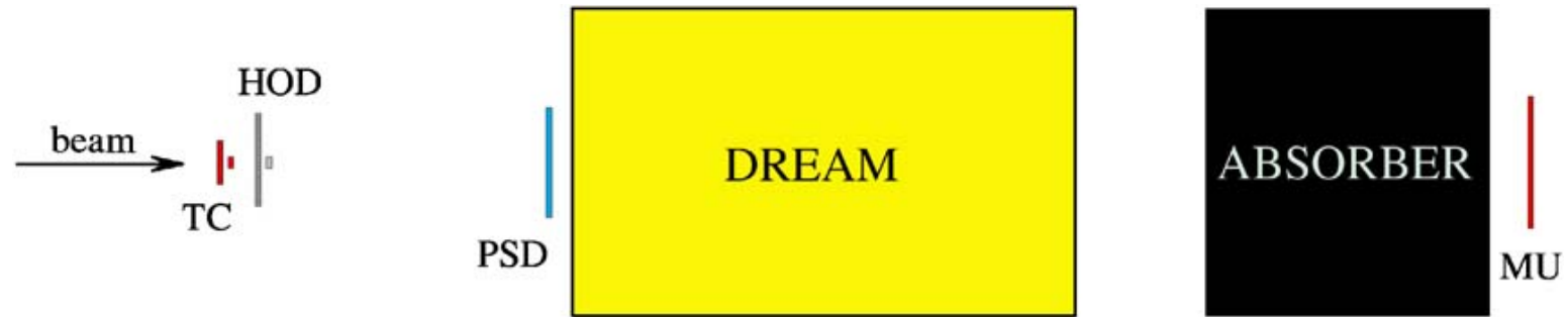
Fig. 4. Schematic view of the experimental setup in the beam line in which the DREAM detector was tested with electrons (see text for details).
